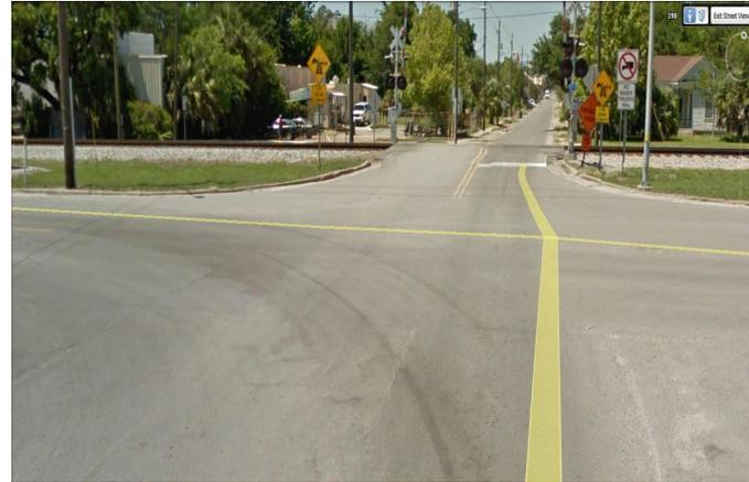
This is the view the Echo Coach driver had as he made a left turn to cross the RR tracks. The severe slope of 45 inches on the far side of the tracks is not visible to the driver as he tried to cross. Additional signage has been added to the tracks since the accident, showing "No Buses-Trucks or RVs". Before the accident, the only signage was Low-boy trucks not to cross (sic).
